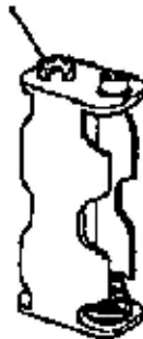
Metal connector riveted to plastic box
