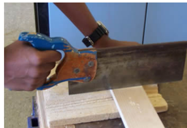
Using a bench hook for sawing.
