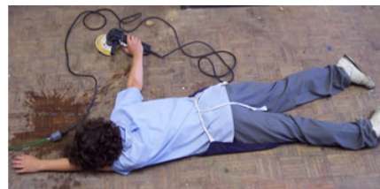
This situation is unsafe, note the trip hazard, unclamped material, power lead wrapped around moving part and the clutter.
