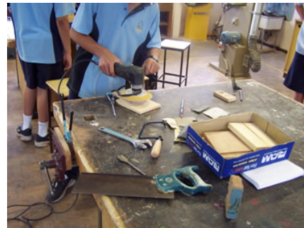
This situation is unsafe, note the trip hazard, unclamped material, power lead wrapped around moving part and the clutter.
